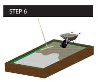
Fill the grid with your chosen aggregate either using a wheelbarrow or direct from a truck. Ensure the truck does not drive on unfilled cells. CORE Drive is designed to be covered by a 10-15mm dressing layer of aggregate making the grid virtually invisible.
