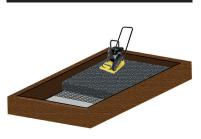
Install membrane and geogrid if required and then the subbase material. Ensure the subbase is well compacted using either a pedestrian roller or vibrating road plate.
